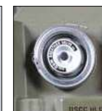
Breather Valve Desiccant
